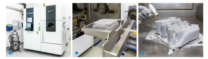
LINK has several of these innovative systems for additive manufacturing (1). At the end of the production process, the powdery »cake« is removed from the machine (2). The freshly manufactured implants are exposed in a special blasting cabin (3). Top: Compilation of LINK products made by additive manufacturing.
