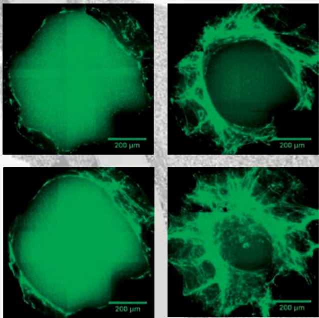
The sequence of pictures shows the pore fill of the TrabecuLink structure under in vitro cell culture conditions.
