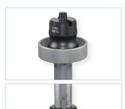
The Assembling Protector for Female Taper (16-0111/01) is placed into the reception of the assembling Table Superior Component.
