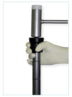
Assemble the elements with two blows of the nonresilient Mallet, using the metal face of the Mallet only.
