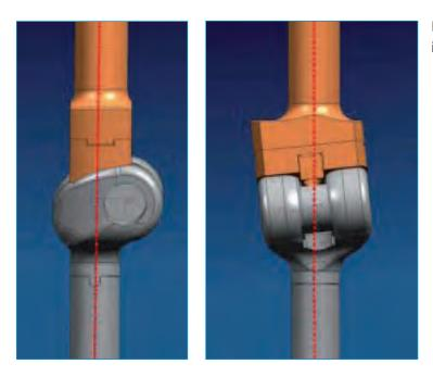
Its use enables taper engagement in axial alignment.
