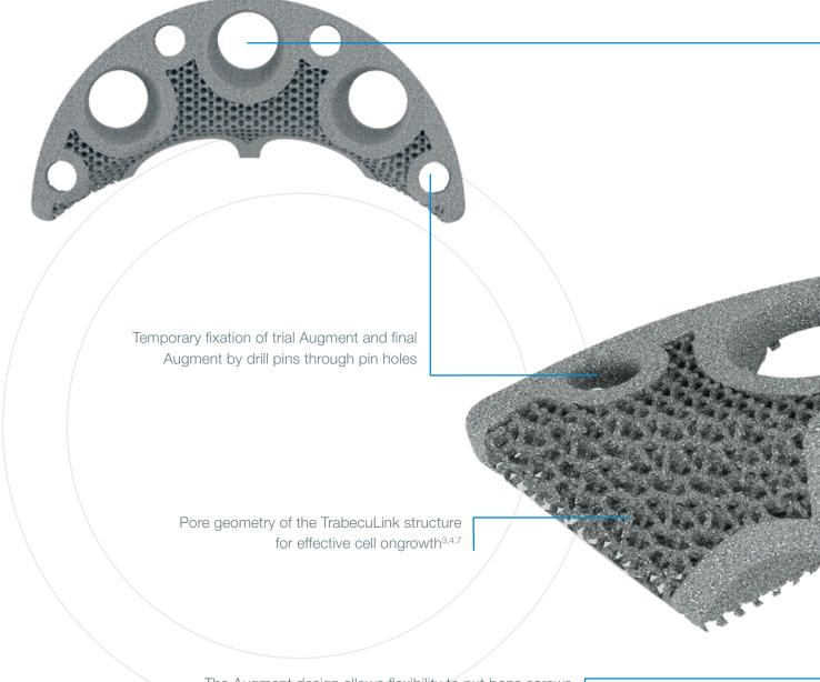
The Augment design allows flexibility to put bone screws through shell and Augment – big recesses allow for great variability in positing the Augment<sup>5</sup>
